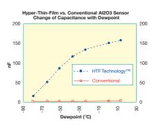
change is quasi linear and its sensitivity to temperature is negligible. The advantages of a linear high capacitance response are: better sensitivity, better repeatability and faster response
