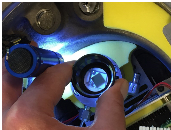
Figure 44 Checking the Mirror Surface
